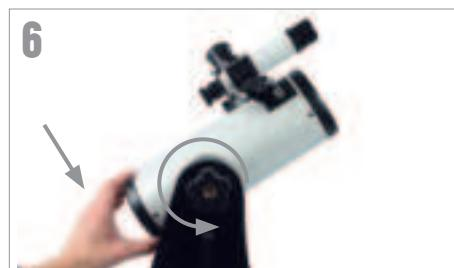
Loosen the altitude lock nut by turning it clockwise and hold the bottom of the tube with your other hand.
