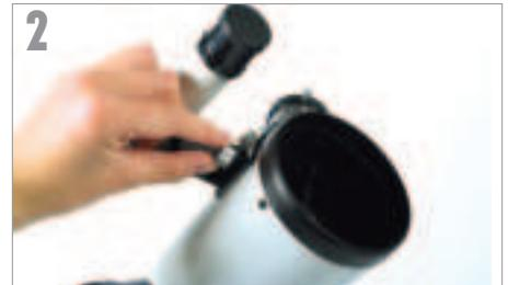
To install the finderscope, remove the nuts on side of tube, place the finderscope bracket over threaded posts and replace the nuts.
