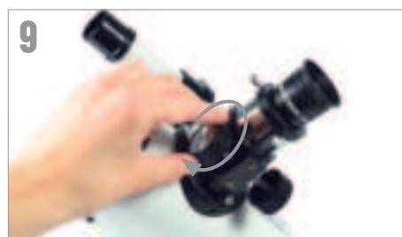
Focus your telescope by turning the two knobs under the eyepiece until you have a sharp image.
