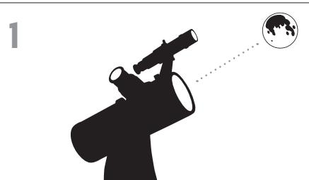
With the Moon visible in the sky, set up your telescope with the 20mm eyepiece installed. Move the telescope so that it is roughly pointing toward the Moon.
