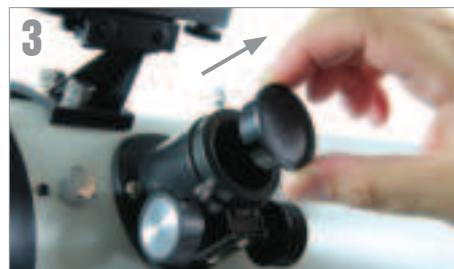
Loosen the thumbscrews on the focuser and remove the focuser cap.
